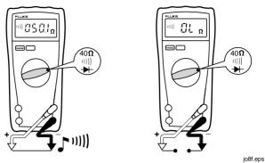
Opens or shorts > 1 ms are detected. Press RANGE momentarily for lead compensation. Press RANGE 1 second to turn the beeper off and place the meter into Lo-Ohms autoranging.
