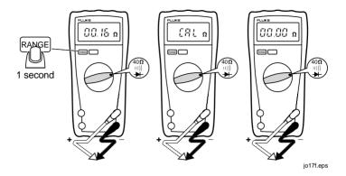
When zero is displayed, compensation has occurred. The meter stays compensated until you change functions.
